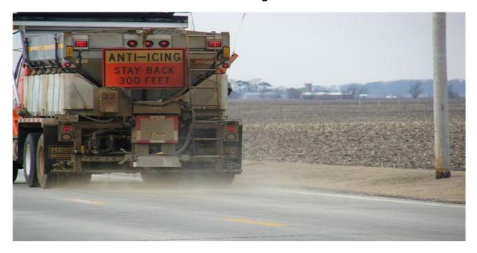
Apply before storm event to prevent Bonding Apply at 20-30 gals / Ln mile(47-71 ltrs / kilometer)\*\* Reduced application rates 30% Reduce application rate for Frost protection - bridges Residual will last 4-6 days Truck and Employee can cover 30% more area Prevents snow & ice bonding – removal easier Increase Manpower & Equipment efficiency Reduced corrosion
