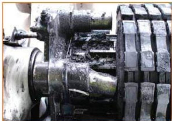
Boeing 767 carbon brake piston failure. Carbon oxidation has led to complete loss of the pressure plate resulting in hydraulic piston collapse.
