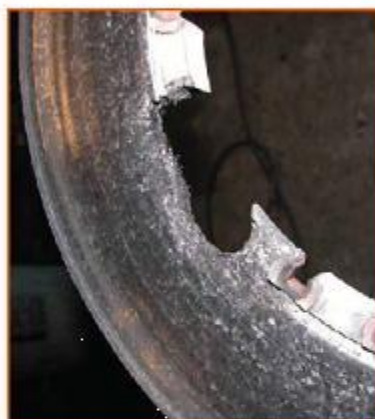
Carbon brake stator oxidation. Carbon oxidation has led to degradation of structural strength and subsequent loss of drive insert.
